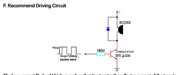
The base current Ib should high enough so that it saturates the collector current of the transistor with the CB load.
