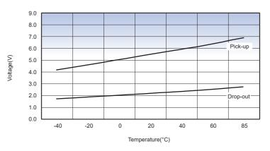
Pick-up Voltage / Drop-out Voltage Curve
