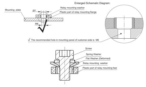
When use M6 screw, the thickness and strength of the washer needs to be guaranteed or it may deform and burst the cover.
