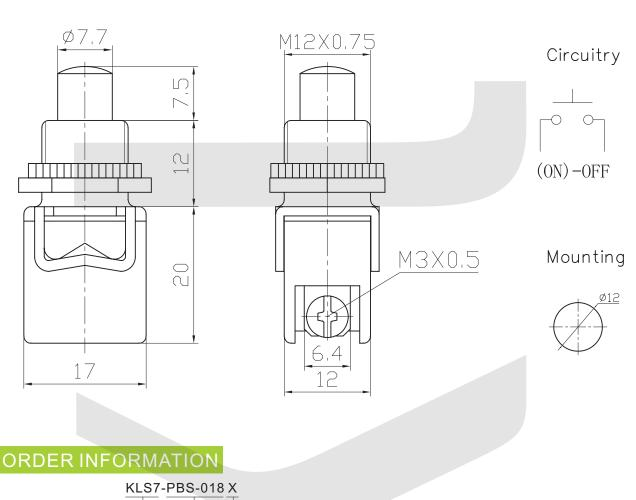
Function: B=ON-OFF C=ON-(OFF) D=OFF-(ON)
